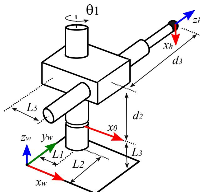
11. According to the DH conventions, we can assign frames to the joints as:
