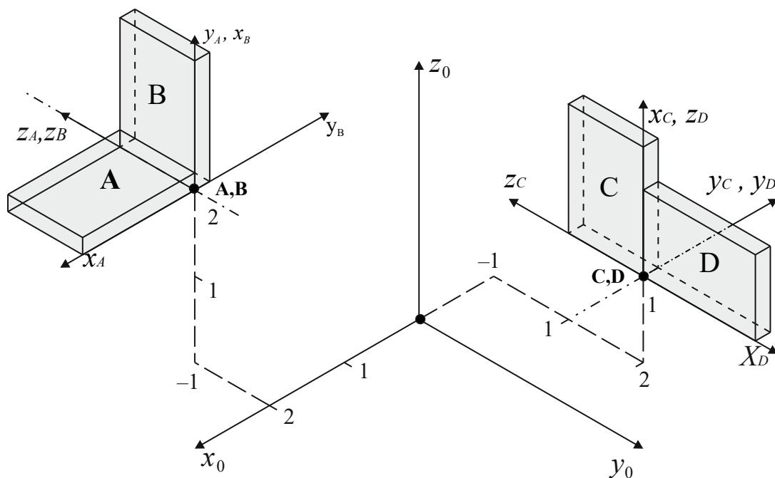
6. The **relative** rotation matrix that displaces object A into the new pose **B** is:
