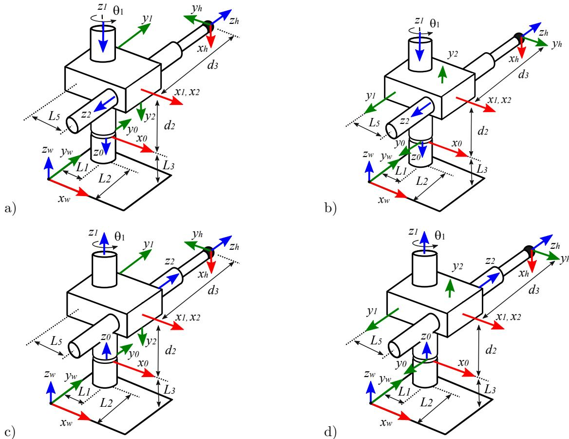
12. The DH parameters of the **spherical** wrist joints:
