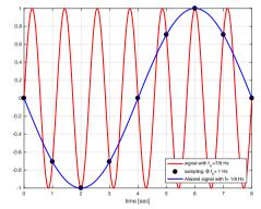
• Note that the frequency of the two sinusoids are 7/8 Hz, 1/8 Hz and sampling frequency  $f_s = 1$  Hz (try to deduce these from the plot). Do you realize any pattern?
