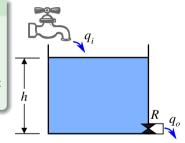
*c<sub>d</sub>*: valve discharge coefficient *a*: valve cross section area
