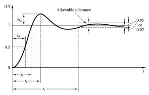
• time required for the response to go from 0 to 100% of its final value.
