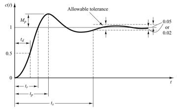
• In this response, the performance indices are usually defined: rise time; peak time; settling time; maximum overshoot; and steady-state error.
