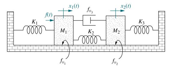
Note that friction shown here is viscous friction. Thus,  $fv_1$  and  $fv_2$  are not Coulomb friction, but arise because of a **viscous** interface.
