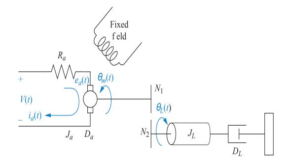
• for a DC motor, mechanical and electrical equations are:
